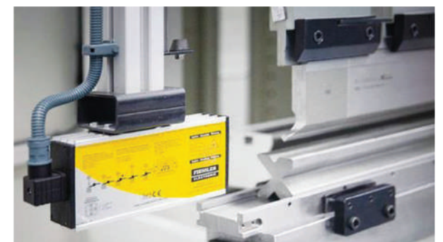
CE Safety system Our machines are designed in accordance with Ce-Norms To ensure your safety with hydraulic, electric, appropriate height covers and laser light curtains. CE safety in tandem Machines are also provided with light barriers
