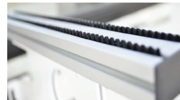
Front support arms with broshes are mounted on a linear guide rall ayatem
